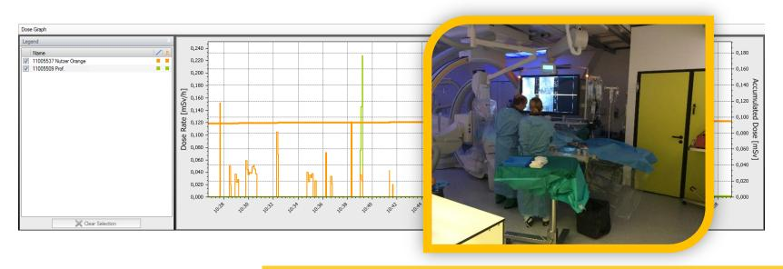
NOTE: MANY TIMES POSITION DIRECTLY BEHIND LEAD SHIELD BETTER PROTECTED SUGGESTION: USE RAYSAFE TO EFFECTIVLY POSITION (E.G. BEHIND OPERATOR)
