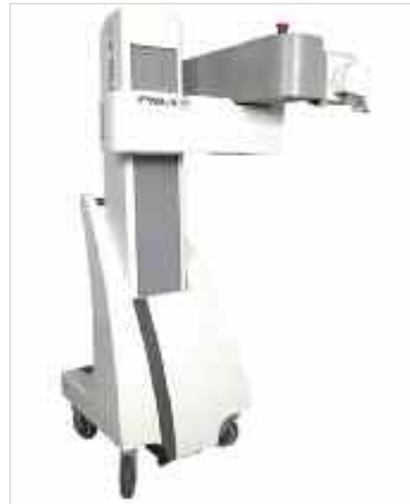
PIGA-CT: a robotic system for the precise placement of needles during image-guided procedures.
